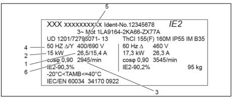
Fig. 6: Motor type plate (example)
